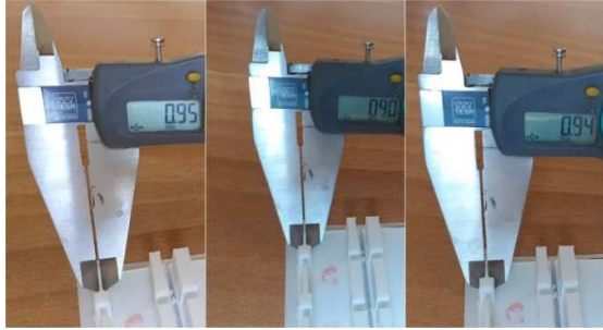
Fig. 2. Measurements taken by digital caliper (with MPE \leq 0.02 mm).
