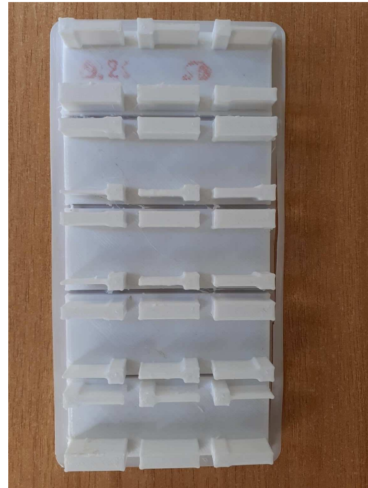
Fig. 1. ISO ASTM 52902-2021 specimen-feature with coarse resolution ribs.
