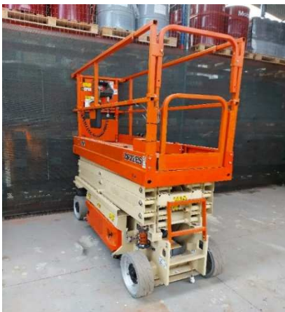
Fig. 3. Nacelle-type auto-lifting platform
