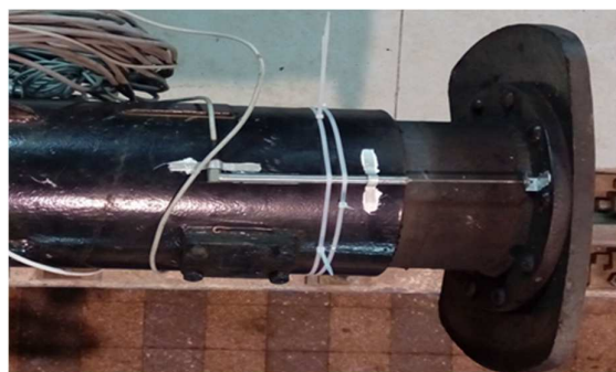
Fig. 7. Mounting the inductive displacement transducer on a buffer.
