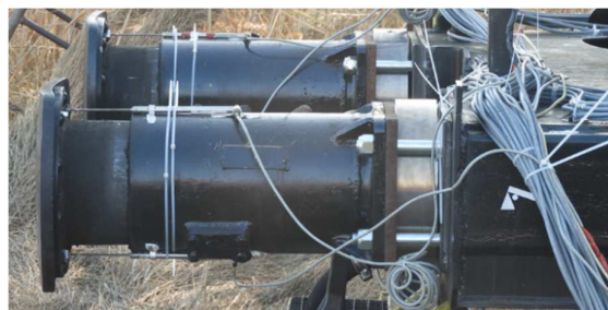
Fig. 8. Mounting the transducers on a buffer.
