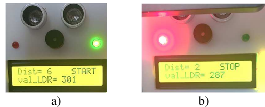
Fig. 13. The values of distance and photoresistor: a) green LED light up, b) a) red LED light up
