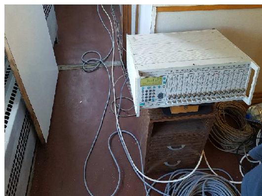
Fig. 3. The data acquisition system from the laboratory wagon
