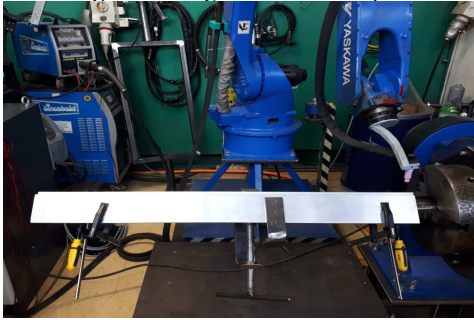
Fig.7. Welding of the stiffened and cooled part
