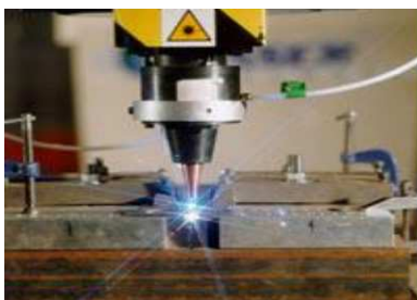
b detail from work space in LBW of carbon steel Fig. 1. Laser welding
