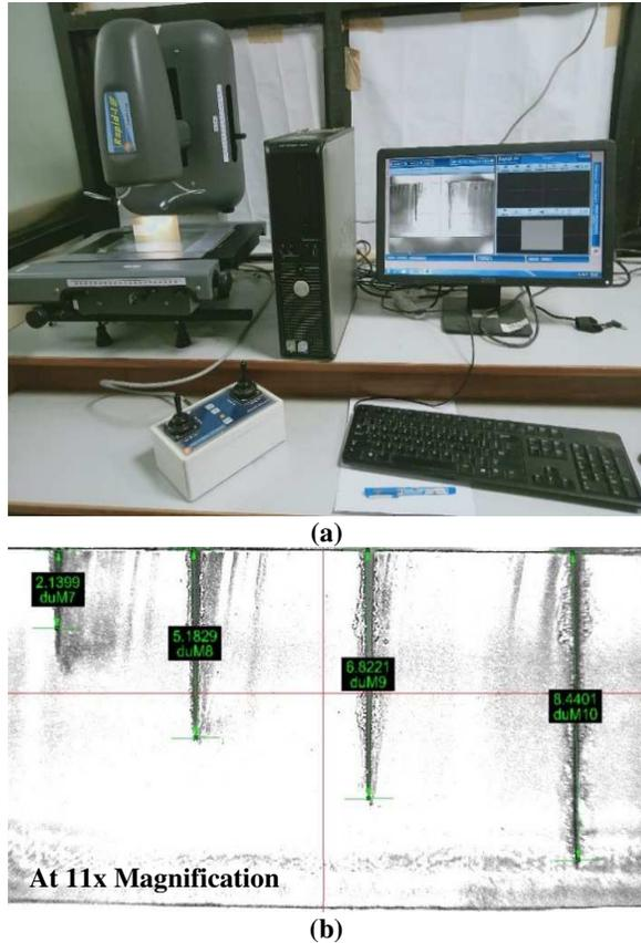
Fig. 4. (a) Vision measuring machine (Rapid-I), (b) Ablation depth at P= 30 W, v=20 mm/s
