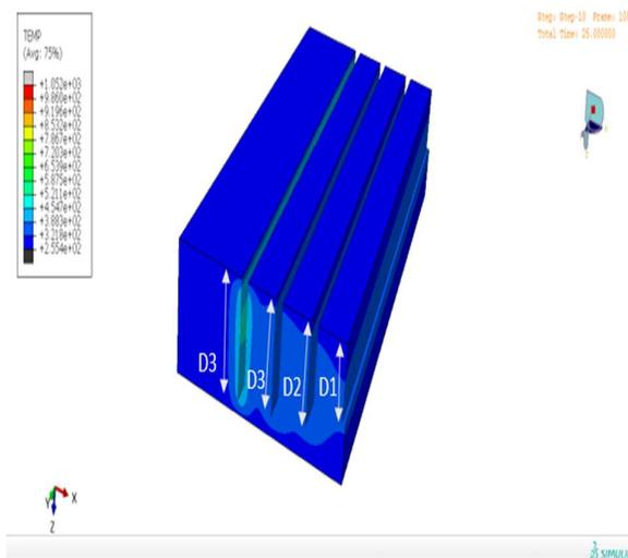
**Fig. 3.** Simulation result of ablation depth in multiple passes at (P=55 W, v= 20 mm/s).
