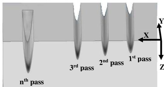
Fig. 1. CAD Model to show multipass laser cutting process.
