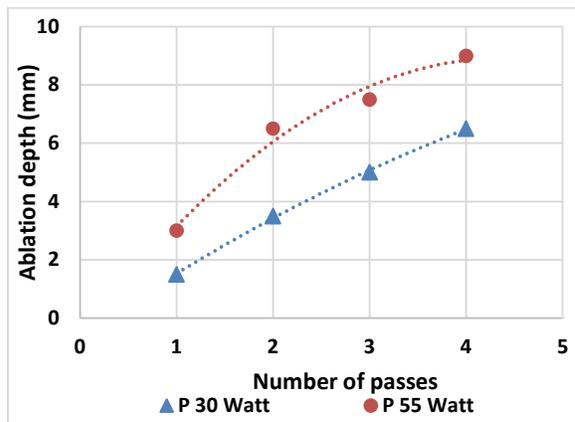
Fig.6. Simulated results of ablation depth in multiple passes at (P=30 W & 55 W).
