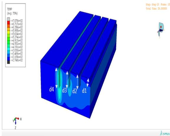
**Fig. 2.** Simulation result of ablation depth in multiple passes at (P=30 W, v= 20 mm/s).
