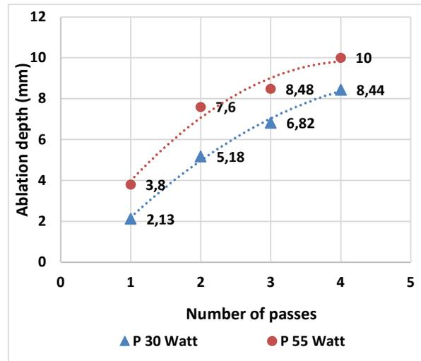
Fig. 5. Experimental results of ablation depth in multiple passes at (P=30 W & 55 W)
