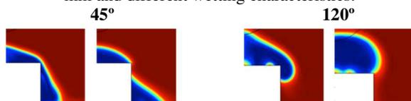
**Fig. 8.** Snapshots of droplet impact on surface with cylindrical roughness with cylinder radius of  $R=2.7$  mm and different wetting characteristics, for  $t = 0.05$  s and  $t = 0.1$  s.
