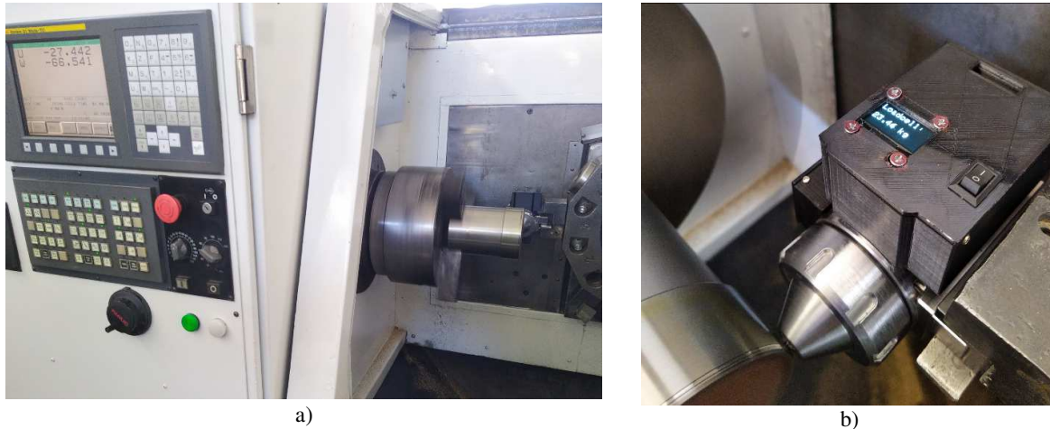
Fig. 2. Setup of the ball-burnishing tool in the CNC lathe turret: a) general view; b) closer view.
