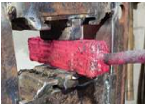
Fig. 2. Bundle of sheet metal strips of different steels during forging.
