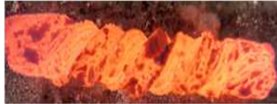
Fig. 4. Image of the strip pack after applying a first twist operation.
