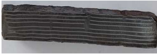
Fig. 3. The bundle of sheet metal strips of different steels before applying the twisting operation (bundle dimensions: 200x22x18.5 mm 3 ).
