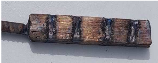
Fig. 1. Bundle of sheet metal strips of different steels assembled by welding (bundle dimensions: 150x20x30 mm 3 ).
