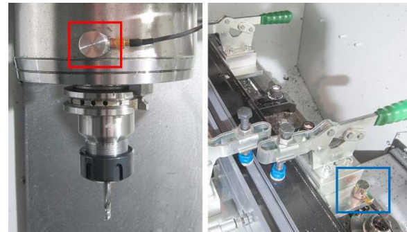
Fig. 5. Detail of placement of two accelerometers: on the spindle in Y-direction (left - red) and on the fixture in Z-direction (right - blue).
