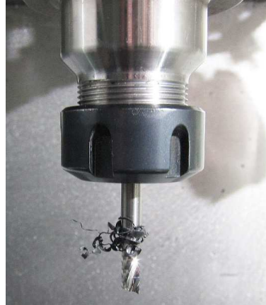
Fig. 14. Detail of accidentally created long chip remaining on the tool after finishing the pocket machining with the strategy S.
