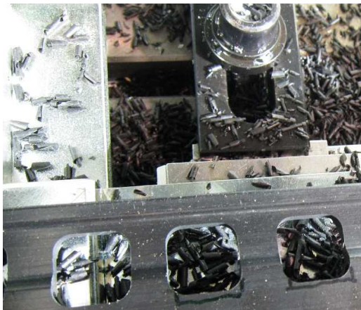
Fig. 13. Detail of the machining setup with created well-segmented chips.
