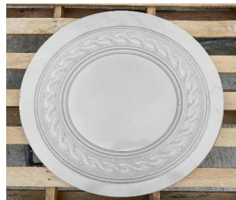
Fig. 6. Thermoplastic mold, ready for use.
