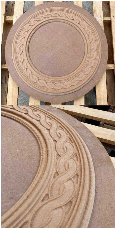
Fig. 2. The frame, created by subtraction method.
