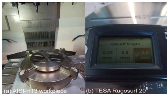
Fig. 2. The experimental setup: the round test piece (a) and the roughness gauge (b).
