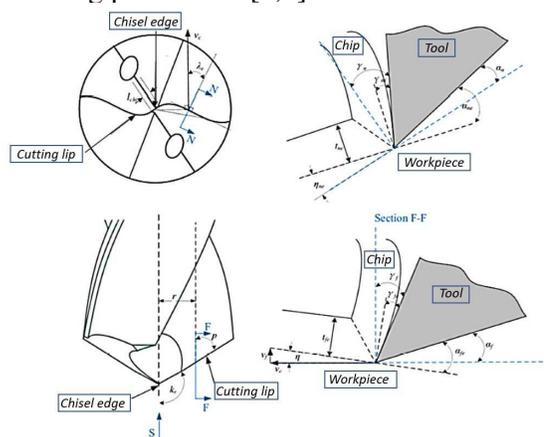
Fig. 1. Schematic view of cutting geometry [8]
