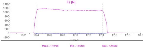
**Fig. 7.** Axial force measured in tests
