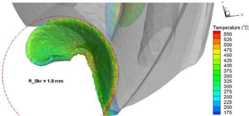
Fig. 11. FEM predicted chips shape
