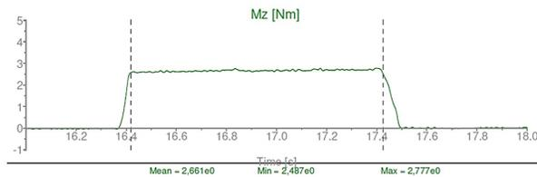
**Fig. 8.** Torque measured in tests
