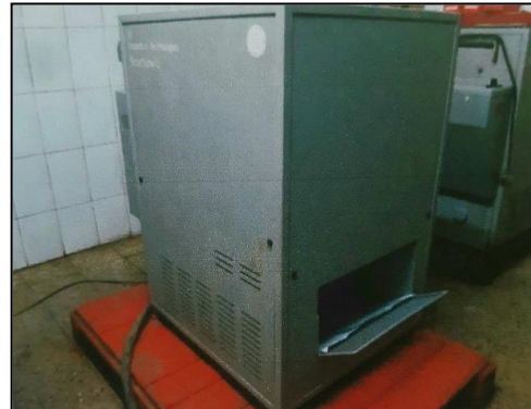
Fig.14. Film processor after exposure to X-rays :a) external and b) internal view
