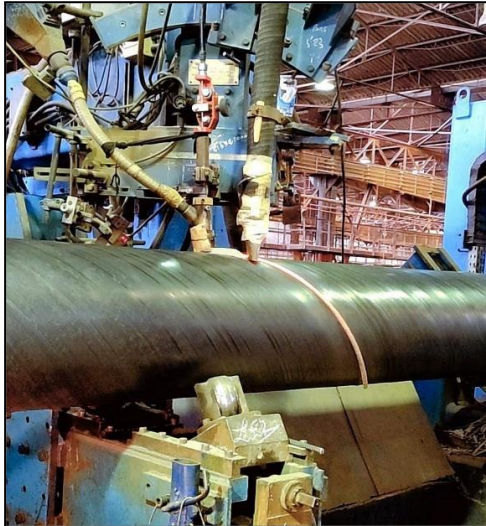
Fig.9. SAW welding (photo taken at ALTUMET).
