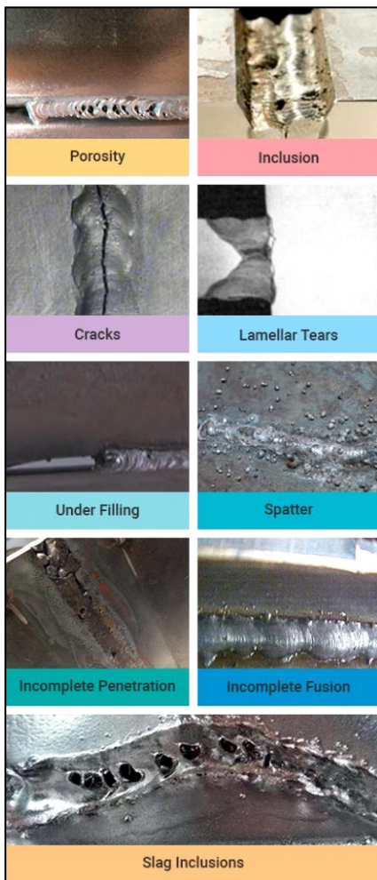
Fig.10. Different types of weld defects [13].
