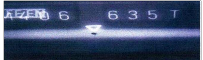
Fig.20. Defect N°5 (isolate blowhole).
