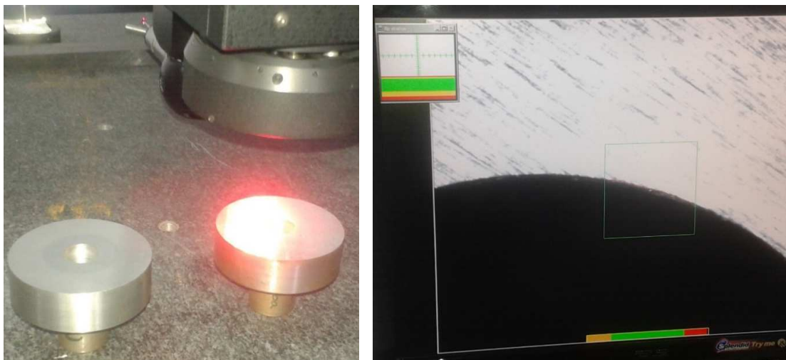
Fig. 5 Interference-fit measured with Werth machine
