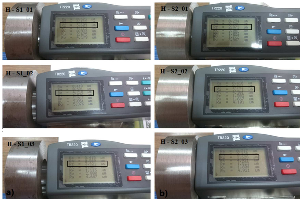
Fig. 3 Hub surface roughness measured with TR220 tester a) the first set (H-S1_01,02,03); b) the second set (H-S2_01,02,03).
