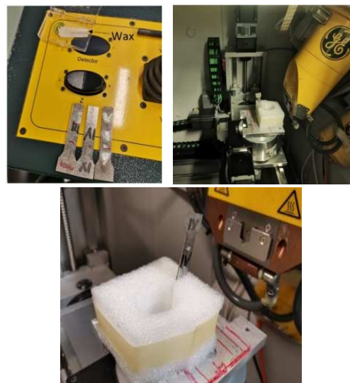
Fig. 5. Sample placed into CT scanner before scanning
