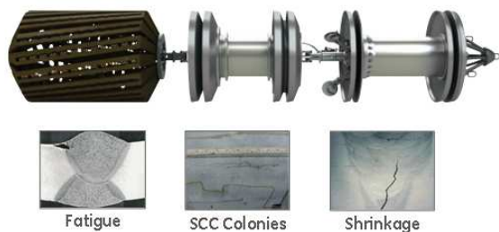
Fig. 2. UltraScan™ CD Plus [8] (top), with mechanical stress induced cracking examples – fatigue, stress-corrosion-cracking (SCC) and shrinkage (bottom).
