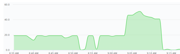
Fig.3. The fluctuation of the Nitrogen Dioxide on a heavy transited road
