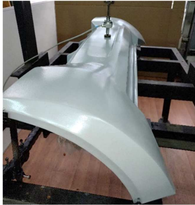
Fig. 3. Rear bumper fascia with central cylindrical surface force application mechanism and transducer. The lateral (off-center) application of force experiment is also conducted for the rear bumper fascia, as seen in Figure 4.
