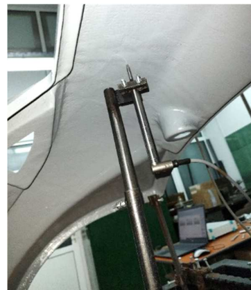
Fig. 2. Displacement transducer placement on the inner side of the investigated car body part
