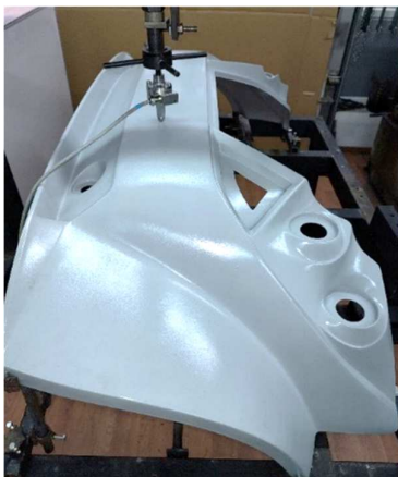
Fig. 1. Front bumper fascia on the test bench with lateral ball point force application mechanism and transducer
