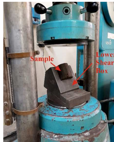
Fig.3. Testing device ready for shear test
