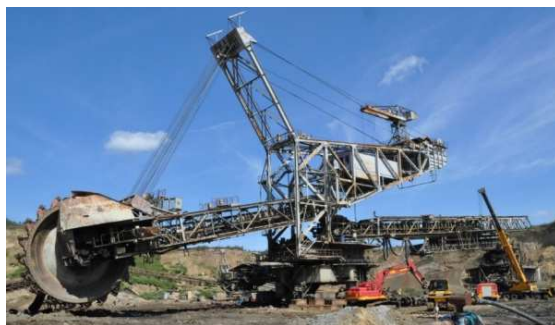
Fig. 3 Bucket wheel excavator type ERc1400-30/7
