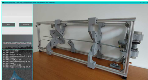
Fig. 4. Graphical user interface, used to control the experimental stand by students in online classes, managed via the Microsoft Teams Share Screen platform
