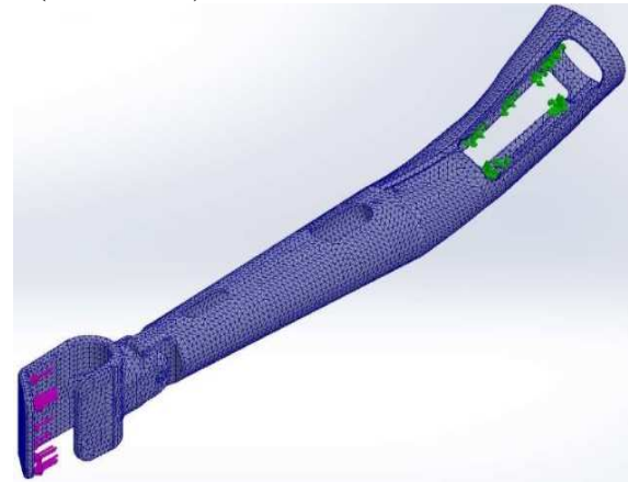
Fig. 5. Finite element model of the distal tensile test used for assessing the mechanical strength of the bicycle prosthesis
