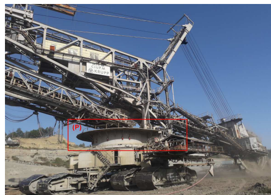
Fig.2. Rotating platform (P) of a bucket wheel excavator
