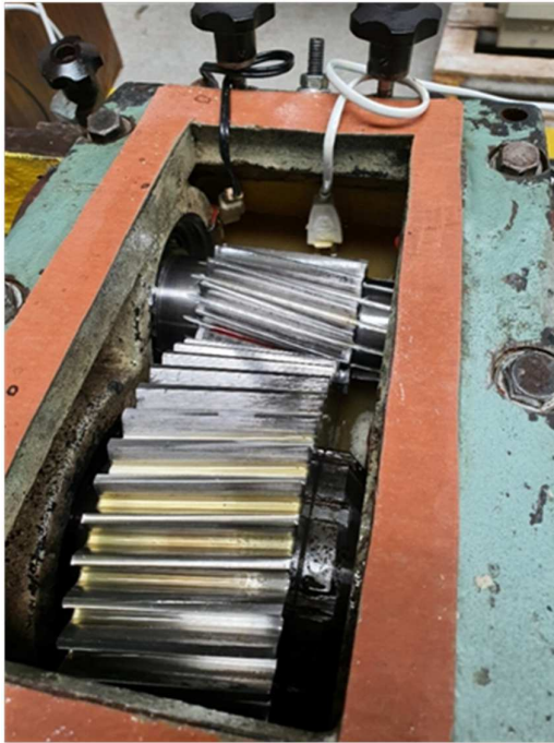
Fig.3. Test housing with electrical resistances in the oil bath
