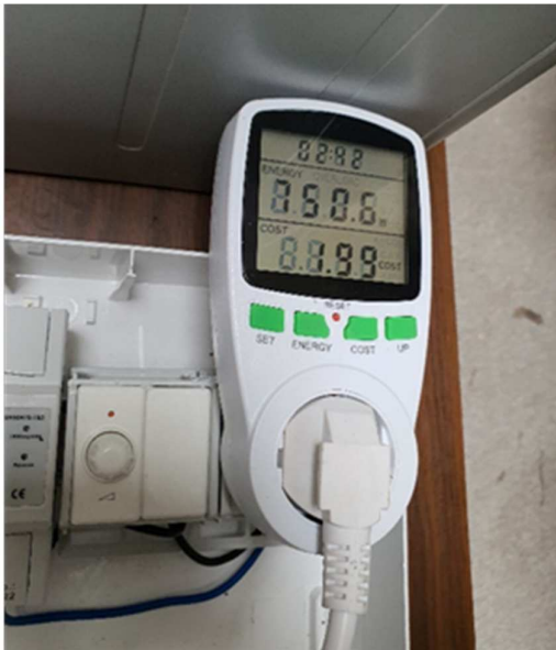
Fig.4. The socket with digital energy meter
