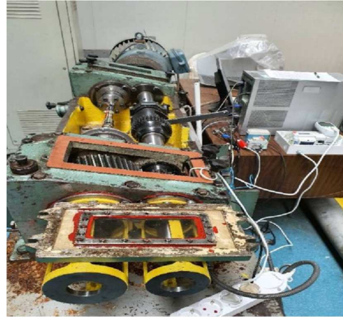
Fig. 1. Mechanical Test bench type FZG with involute gear systems
