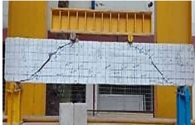
Fig. 10: Preformed crack beam
