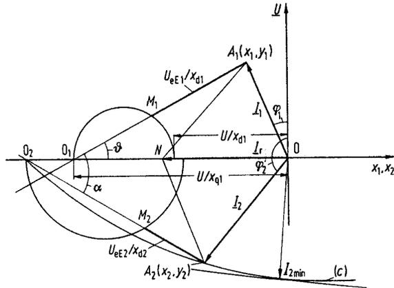
Fig. 3. Phasor diagram for synchronous machines with salient poles
