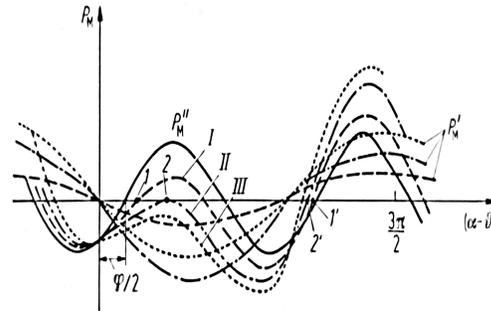
Fig. 4. The equivalent characteristics  $P_M(\alpha - \theta)$
