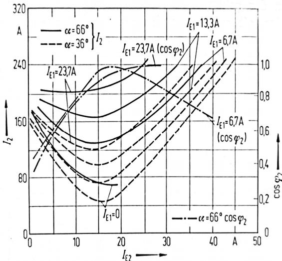
Fig. 7. Curves  $I_2(I_{E2}), \cos \varphi_2(I_{E2})$  for  $I_{E1}=\text{const.}, \alpha=\text{const}$
