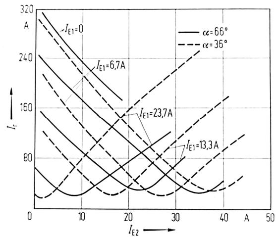
Fig. 8. Curves  $I_r(I_{E2})$  for  $I_{E1}=\text{const.}, \alpha=\text{const}$
