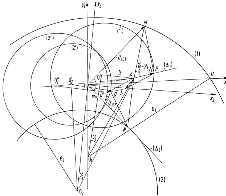
**Fig. 1.** Geometrical locus curves for two coupled synchronous machines at  $P_{M1}=\text{const.}$ ,  $\alpha=\text{const}$
