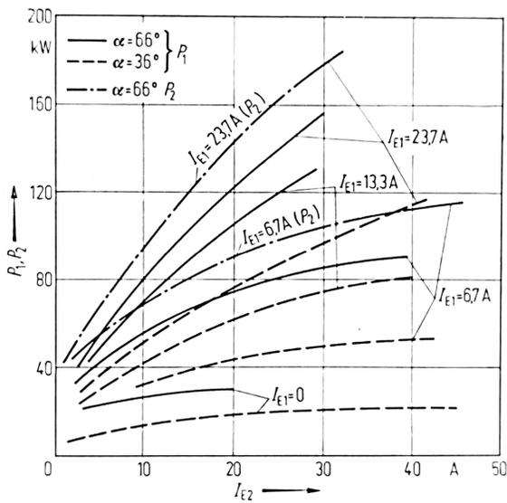
Fig. 6. Curves  $P_1(I_{E2}), P_2(I_{E1})$  for  $I_{E1}=\text{const.}, \alpha=\text{const}$
