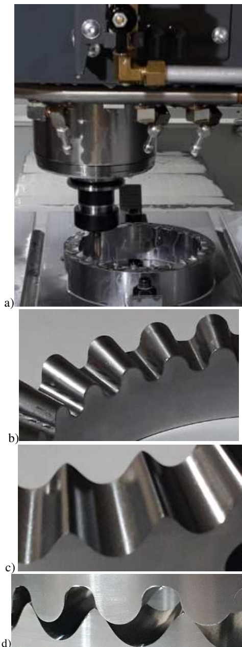
Figure 20. CNC machining center for milling gear teeth with a finger mill (a), internal gear wheel (b) external gear wheel (c), meshing gears (d).
