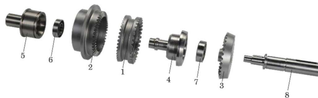
Fig.4. The components of the precessional node, presented with the satellite wheel detachably assembled on the counter-satellite semi-axis with axial floating and tangential sliding (exposing the physical components – manufactured) [2]
