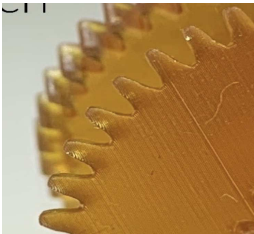
Fig.8. Imperfections in the printed gears
