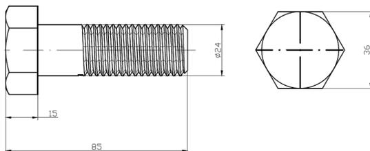
Fig.1. The specimen drawing
