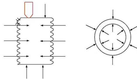
**Fig.8.** Pattern contraction during printing
