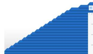
Fig.4. The slicing of an inclined plane
