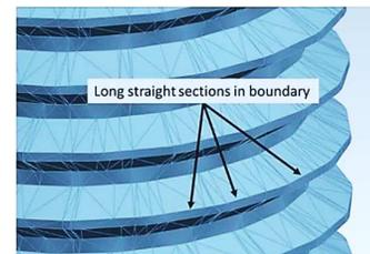
Fig.3. Linearizing the geometry of a CAD drawing into an STL file
