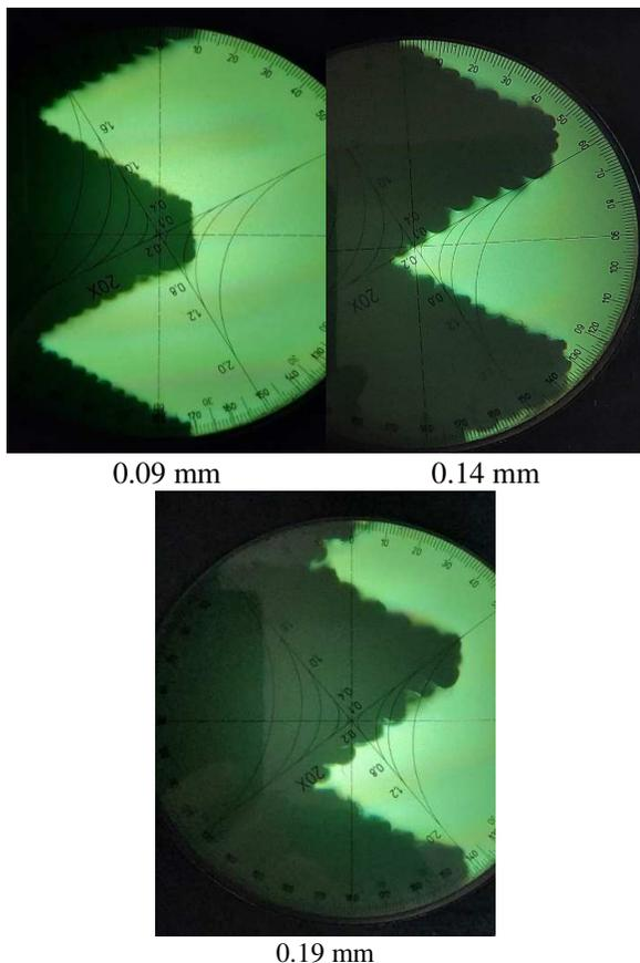
Fig.10. View of M24 screw using the profile analyser
