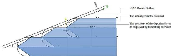
**Fig.6.** Offset sketch between the ideal geometry and the printed one due to the deposition of the middle layer
