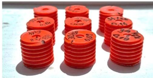
Fig.13. 3D printed parts with flank correction
