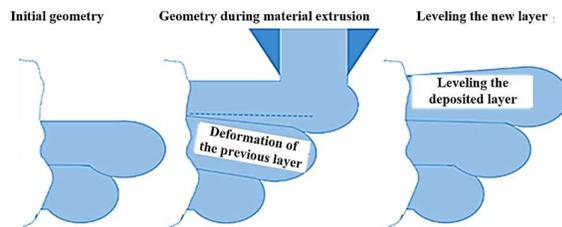
**Fig.9.** Deformation and levelling of the layer during extrusion
