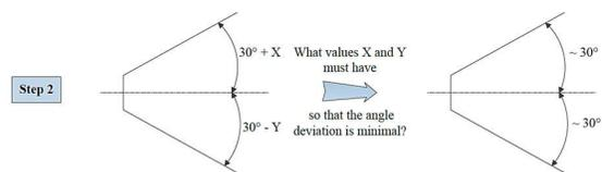
Fig.12. Presentation of the proposed angle compensation method
