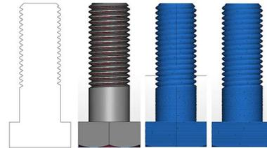
Fig.2. Sketch of the model, CAD model, STL
