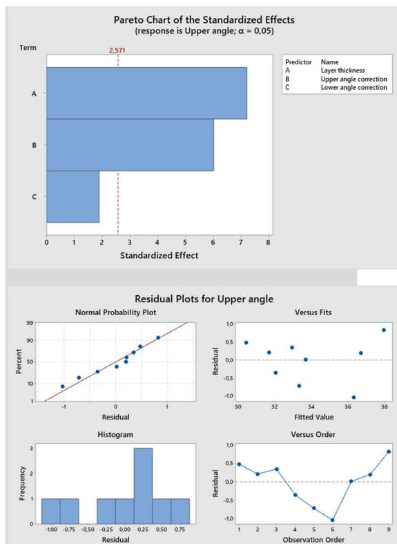
Fig.15. Rapport of regression analysis generated by Minitab software for "Upper angle"
