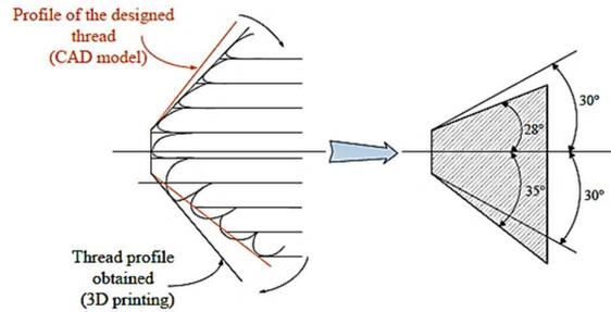
**Fig.7.** Pattern contraction during printing
