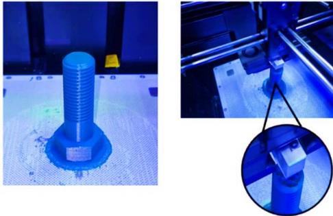
**Fig.5.** The screw during the 3D printing process
