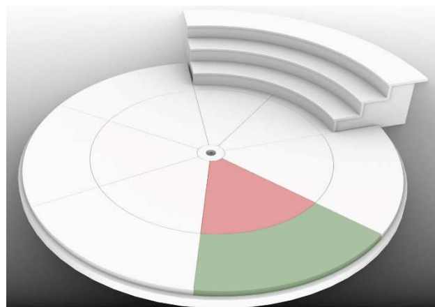
Fig.7. Elements whose mold is made of plywood
