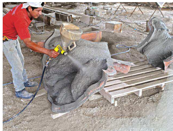
Fig.9. The image shows the process of spraying layers of concrete mixture on an uneven surface using GFRC technology [15]
