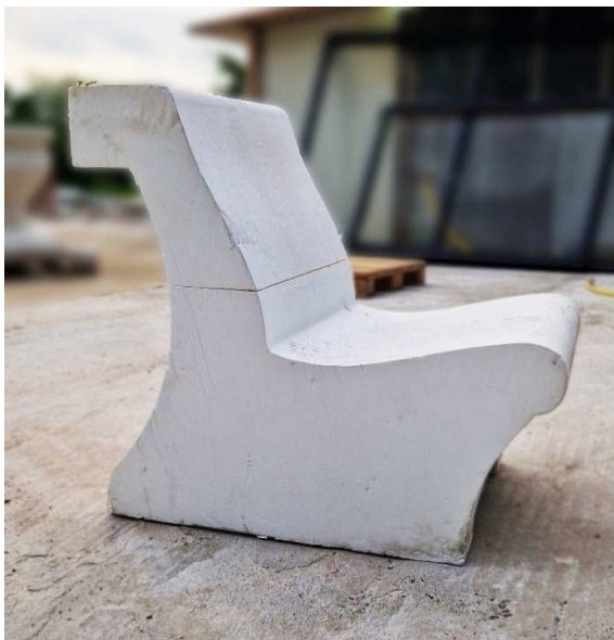
Fig.6. Styrofoam model milled on a CNC router
