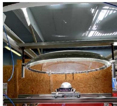
Fig.1. Vertical CSE furnace from PROMES-CNRS
