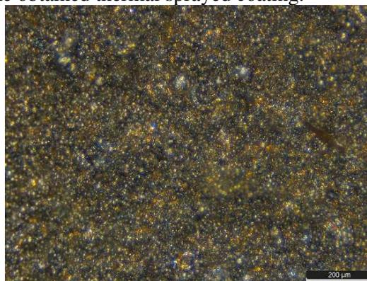
**Fig.3.** Microscopic image of the NiCrAlY thermal sprayed sample
