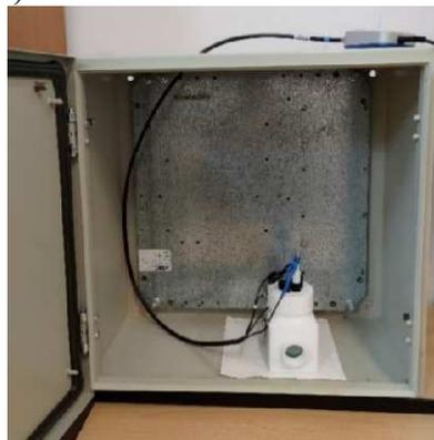
**Fig.4.** Standard cell used for the electrochemical tests
