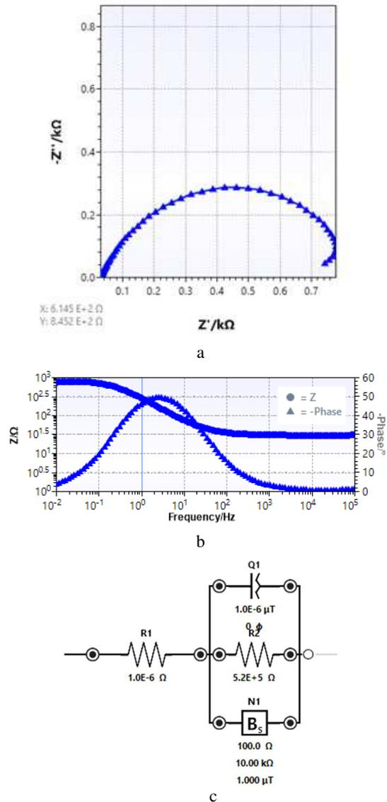
Fig.7. EIS data as Nyquist plots (a), Bode plots (b) and model equivalent electrical circuit for the steel substrate (c)
