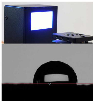
**Fig.5.** Setup used for the wetting behavior analysis
