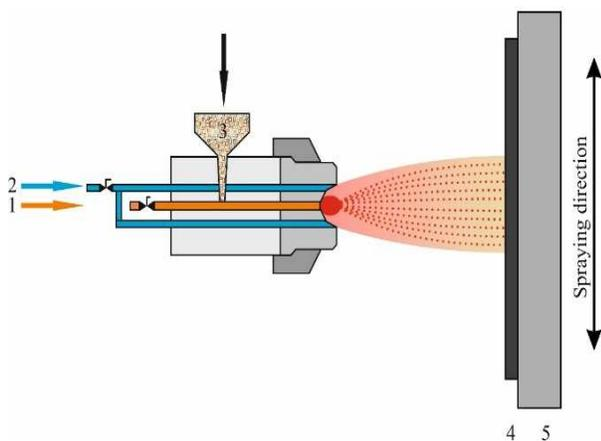
**Fig.2.** Thermal spraying installation principle.
