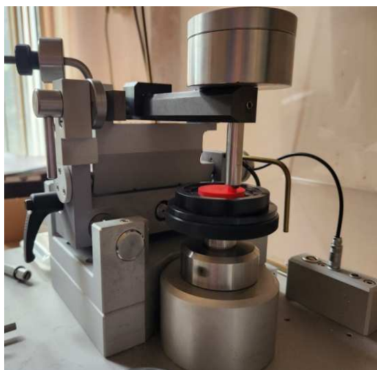
Fig.2. The test machine used to determine the sliding coefficient of friction
