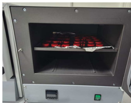
Fig.4. Oven used for applying the heat treatment
