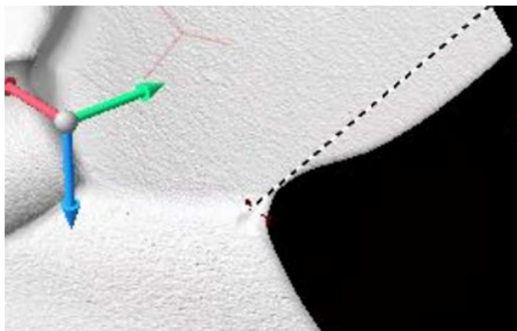
Fig.7. CT scan of rebuilt geometry, visible porosity in the filled area
