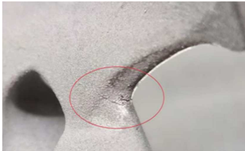
Fig. 6. Titanium Grade 5 component with hairline crack
