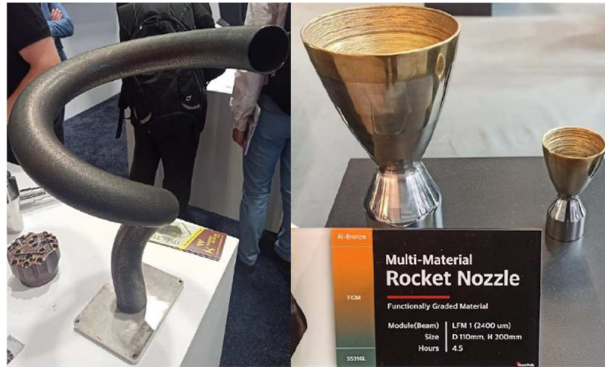
Fig. 1. (left) DED freeform design, without support structures, (right) DED multi-material structures, own pictures from Formnext Frankfurt, 2022
