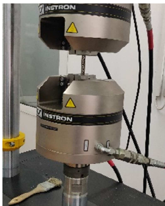
Fig. 5. Instron 8801 set-up for tensile test
