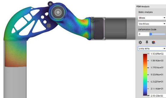
Fig. 3. FEM analysis of the stresses on the redesigned component
