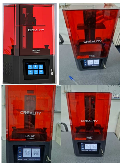
Fig. 3. 3D printer used for DLP technique.
