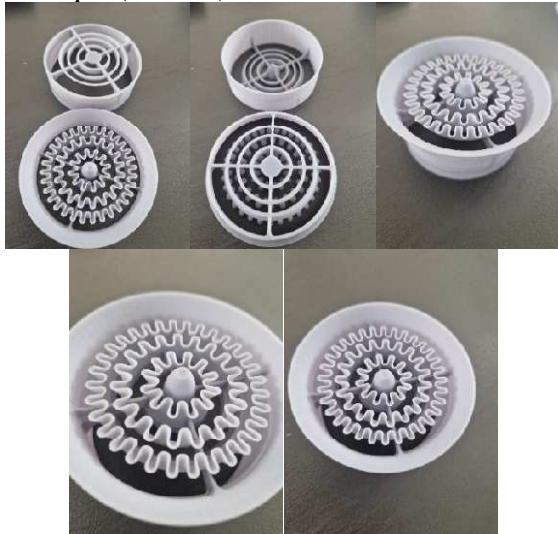
Fig. 9. The air diffuser 3D printed with DLP technique – second iteration.
