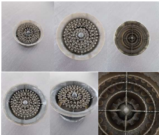
Fig. 10. The air diffuser 3D printed with SLA technique.
