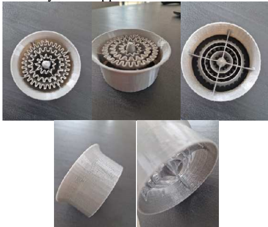
Fig. 5. The air diffuser 3D printed with FDM technique.
