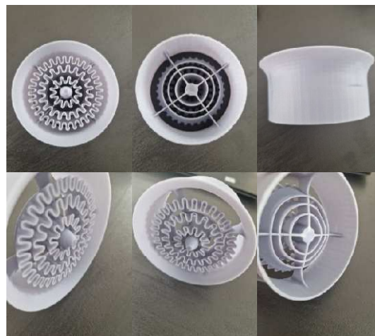
Fig. 7. The air diffuser 3D printed with DLP technique.
