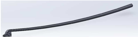
Fig. 7. – 3D model of the bow rod (hexagonal profile).
