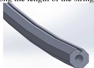
Fig. 1. Variant 1 - hexagonal section with a "T" groove.
