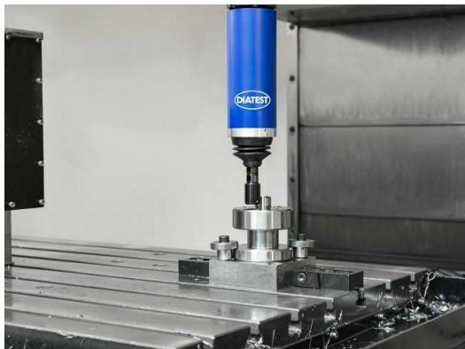
Fig. 2. Installation of measurement system on the CNC toolholder.[22]
