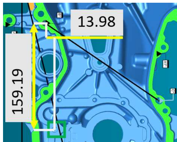
Fig. 5. Drawing measurement coordinate system ABC and reference P coordinates.
