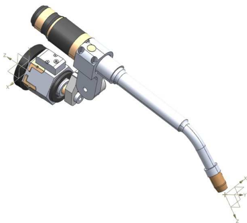
Fig. 5. Defining GMAW gun coordinate systems
