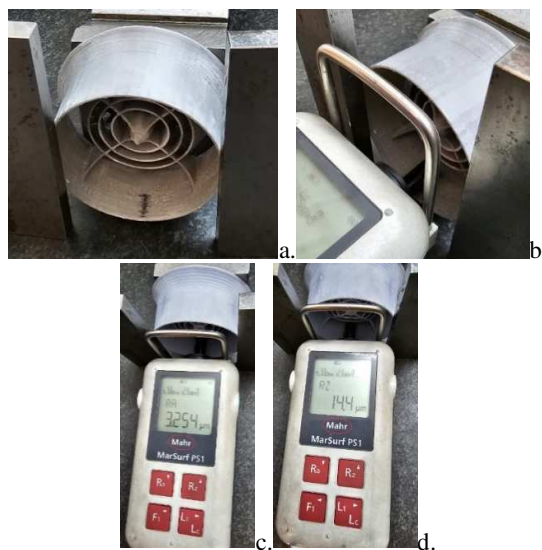
Figure 3. a. Positioning of the printed diffuser in order to take the roughness measurements; b Positioning of the MarSurf PS1 equipment; c. Ra parameter measurement; d. Rz parameter measurement.
