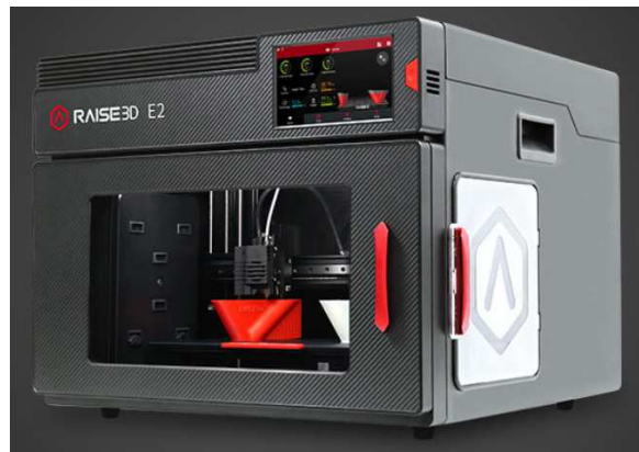
Fig.11. The desktop 3D printer (RAISE 3D E2) used in this work
