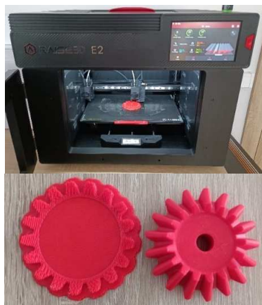
Fig.12. The desktop 3D printer (RAISE 3D E2) used in this work
