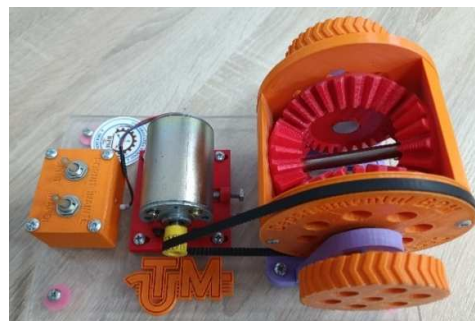
Fig.14. Final working assembled differential transmission
