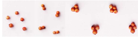
Fig.15. The seeds used to calibrate the transducer: a) a seed; b) group of 2 glued seeds; c) group of 3 glued seeds; d) group of 4 glued seeds
