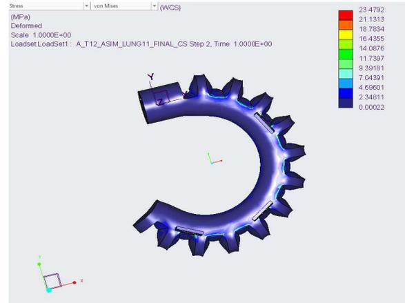
**Fig.14.** Predicted behaviour of the pneumatic actuator with built-in flanges; Applied pressure is 0.45MPa
