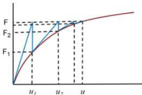
**Fig.3.** Application of the stress force in the nonlinear static analysis; F represents the force increment; u - deformation increment
