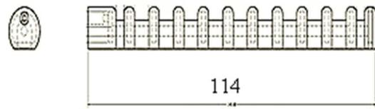
**Fig.8.** Bidimensional sketch of the M2 pneumatic actuator
