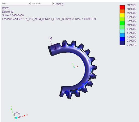
**Fig.13.** Predicted behaviour of the pneumatic actuator with flanges. Applied pressure is 0,4 MPa
