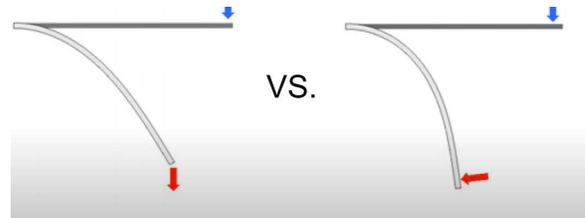
**Fig.4.** The difference between force application in the case of linear static analysis vs. non-linear statics
