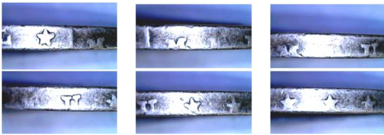
Fig.5. The lettering misaligned position
