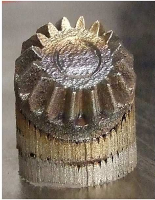
Fig. 3 Sewing machine gear manufactured using SLM process [51]
