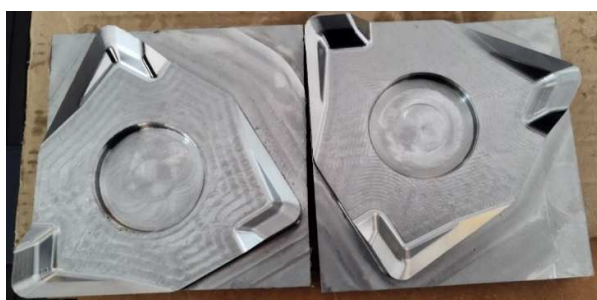
Fig.14. Two different surface quality of the part
