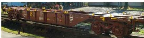
**Fig.3.** Platform wagon with highlighting of attachment points, source Đuro Đaković website
