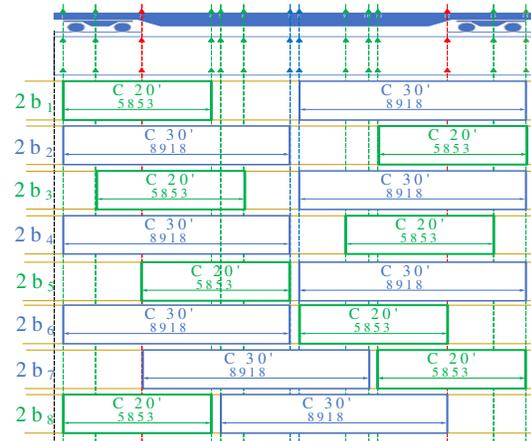
**Fig.10.** Wagon loaded at partial capacity with two container types 20' and 30' (in mm)
