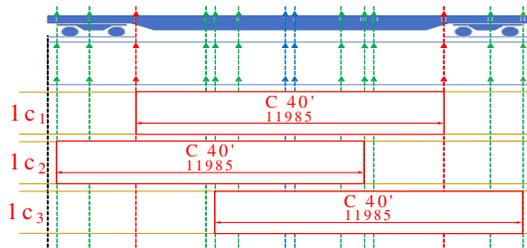
**Fig.8.** Wagon loaded at partial capacity with 40' type container (in mm)
