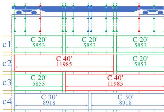
**Fig.5.** Wagon loaded to maximum capacity (in mm)
