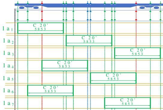
**Fig.6.** Wagon loaded at partial capacity with 20' type container (in mm)
