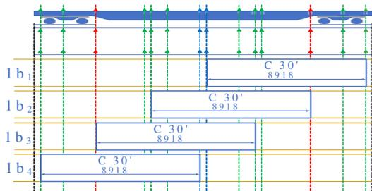
**Fig.7.** Wagon loaded at partial capacity with 30' type container (in mm)
