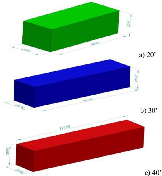
Fig.14. 3D container models (in mm)
