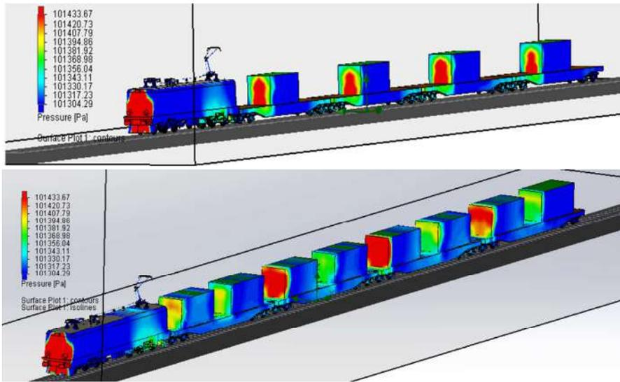
**Fig.18.** Pressures exerted on the front fenders of the train
