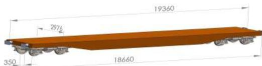
Fig.13. 3D model platform wagon Sgnss (in mm)
