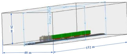
**Fig.16.** Volume of air delimited for flow
