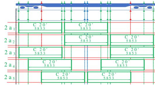
**Fig.9.** Wagon loaded at partial capacity with two 20' container type (in mm)
