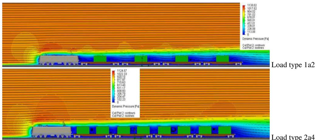
**Fig.17.** Dynamic air pressure distribution in the longitudinal plane of the train
