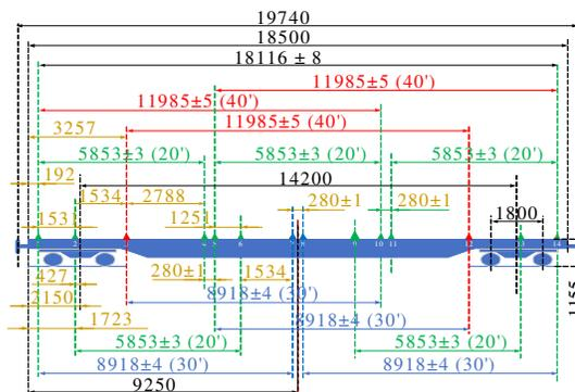
**Fig.4.** Arrangement of attachment points (in mm)
